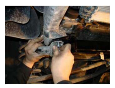
4. Slide the steering brace around the anti-sway bar and push everything together back against the frame while guiding the new sector nut through the hole in the brace flange. Install the new 10-1.5 x 40mm bolts, lock washers and flat washers - make sure the hole in the flange is centered around the new sector shaft nut - then tighten to 36 lb/ft. Retighten the anti-sway bar link nuts.
