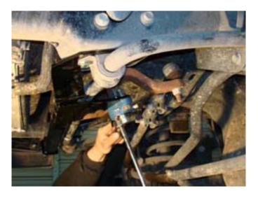
6. Install the 7/16-14 x 2 bolts with flat washers on both sides and nylon locknuts, torque to 75 lb/ft.
