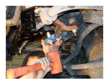
5. Install the bearing block on the the new sector nut. It is a tight slip fit, a soft face hammer may be required to tap the bearing into place.
