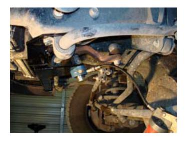
8. To complete the job, grease the bearing block.
