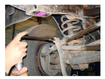
3. Remove sway bar bushing mount bolts, 15mm socket required. Drop anti-sway bar down and loosen sway bar link nut until flush with the end to ease installation.
