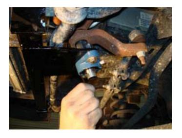
7. Tighten set screws in the collar of the bearing block
