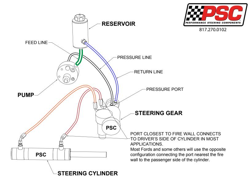
HOSE ROUTING FOR STEERING GEAR BOX / CYLINDER APPLICATION
