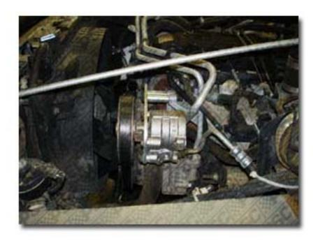
This kit does offset the pump out board towards the drivers fender more and does require moving the windshield fluid bottle a little. This particular vehicle has aftermarket fenders and the windshield fluid bottle was removed.
