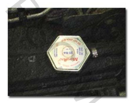
With this particular vehicle we chose to remove the overflow bottle and install a 20# cap. We have had no issues at all by doing this. Being a Texas vehicle, 110 degree days have not been a problem, nor has high altitude driving. Also by going to a higher pound cap you increase the boiling temp. (old racers trick)
