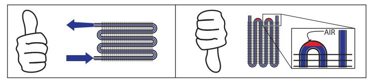
"Tank" type coolers (like a radiator) are a little more forgiving and offer one additional mounting option. The first option is the same as is recommended for the "tube" type cooler - the main tubes, or tanks, should run horizontally with the fluid entering the lower tank and exiting the top. The alternative is to mount the cooler so that the ports are pointed up. Since all the cooling rows are tied together at each tank, air should be able to exit the cooler using either mounting method.
