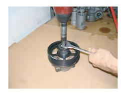
Always use an automotive power steering pulley installer for pulley installation.
