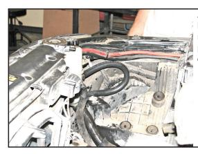
Again, ensure that a loop of sufficient radius is used to prevent any kinking of the hose.
