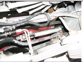
Ensure that a radius exists in the line large enough to prevent hose collapse.
