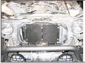
Reinstall items removed during installation then bleed the power steering system according to the enclosed bleeding instructions.
