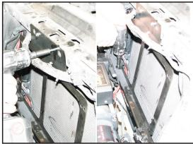
Using the included self-drilling, self-tapping screws install the cooler bracket.
