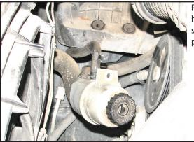
Remove the bolt holding the power steering reservoir in place.
