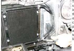
The line from the radiator should go into the bottom of the cooler. The other line should come from the top port of the cooler and go into the transmission return line.
