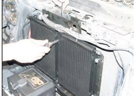
It may be necessary to remove the top 2 screws to gain access to the back of the bracket for mounting the coolers.
