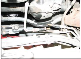
The upper line is the return to the transmission. Cut in the center of the hose. Install two "hose menders."
