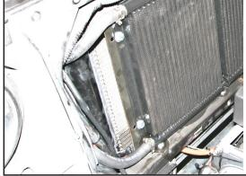
The hose from the steering gear should go into the lower port of the cooler. The upper port should connect to the reservoir.
