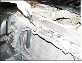
Take the wire loom loose from the header panel.
