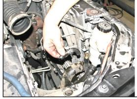
Cut the 90 degree bend from the power steering return line. Insert a "hose mender" into the remaining hose.
